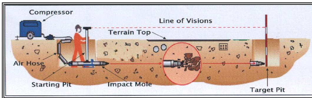
Figure 2: The schematic of impact moling
